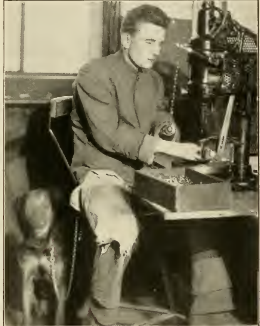
Vertical Thread Cutting Machine, Operated by Blind Worker With One Arm and Paralyzed Right Hand. Knee of Right Leg is Used to Prepare Part to be Threaded
